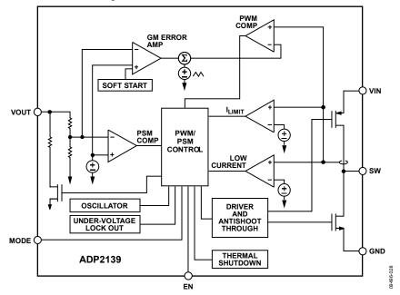
Figure 34. ADP2139 Functional Block Diagram
