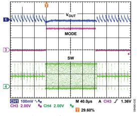
Figure 31. Mode Transition from PSM to PWM to PSM,  $V_{OUT} = 1.8 V$
