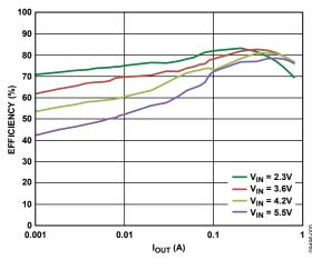
Figure 5. Efficiency vs. Load Current, Across Input Voltage,  $V_{OUT} = 0.8 V$ , PSM Mode
