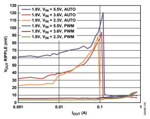
Figure 32. Vout Peak-to-Peak Ripple vs. Output Current, Vout = 1.8 V
