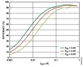
Figure 8. Efficiency vs. Load Current, Across Input Voltage,  $V_{OUT} = 3.3 V$ , PWM Mode
