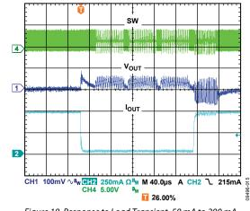
Figure 18. Response to Load Transient, 50 mA to 200 mA,  $V_{OUT} = 1.8 V$ , Automatic Mode
