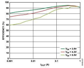
Figure 7. Efficiency vs. Load Current, Across Input Voltage,  $V_{OUT} = 3.3 V$ , PSM Mode
