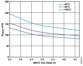
Figure 16. RDSON NFET vs. Input Voltage, Across Temperature
