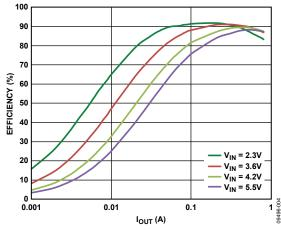
Figure 4. Efficiency vs. Load Current, Across Input Voltage,  $V_{OUT} = 1.8 V$ , PWM Mode
