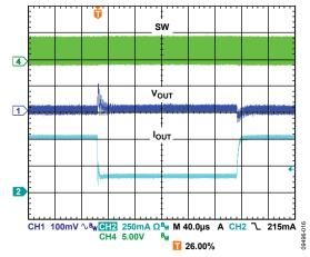
Figure 19. Response to Load Transient, 150 mA to 500 mA, V<sub>OUT</sub> = 0.8 V, PWM Mode
