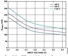
Figure 15.  $R_{DSON}$  PFET vs. Input Voltage, Across Temperature
