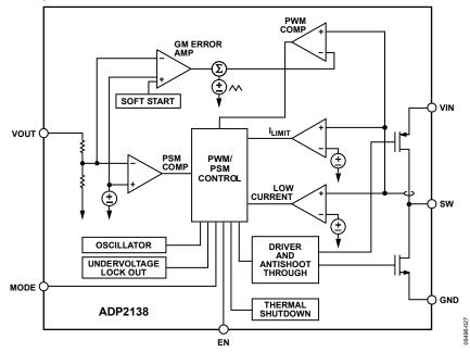
Figure 33. ADP2138 Functional Block Diagram
