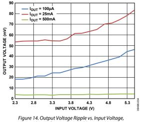
Across Output Current,  $V_{OUT} = 1.8 V$
