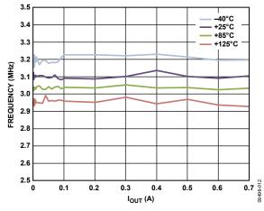
Figure 12. Frequency vs. Output Current, Across Temperature,  $V_{OUT} = 1.8 V$ , PWM Mode
