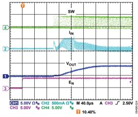
Figure 28. Startup,  $V_{OUT} = 0.8 V$ ,  $I_{OUT} = 10 mA$
