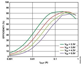
Figure 6. Efficiency vs. Load Current, Across Input Voltage,  $V_{OUT} = 0.8 V$ , PWM Mode
